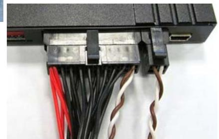
**Anschluss an das Kombinationsinstrument / *Connection to the combined instrument***
