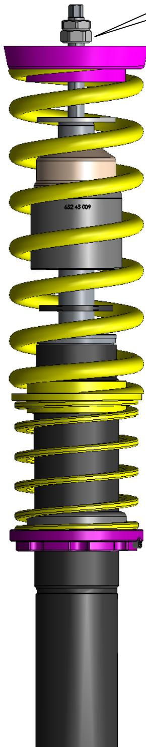
Install the factory top mount and secure it with the supplied nuts. Tightening torque for the piston rod nut is 20 Nm (15 ft-lb). The strut unit has to be installed according to manufacturers instructions settings regarding tightening torque and fixing specifications.
