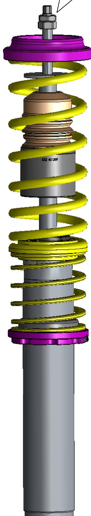
Cut off the dustcover from spring perch on the dashed line. The dust cover is no longer needed.
