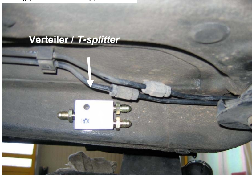
Montageposition 4 / Assembly position 4
